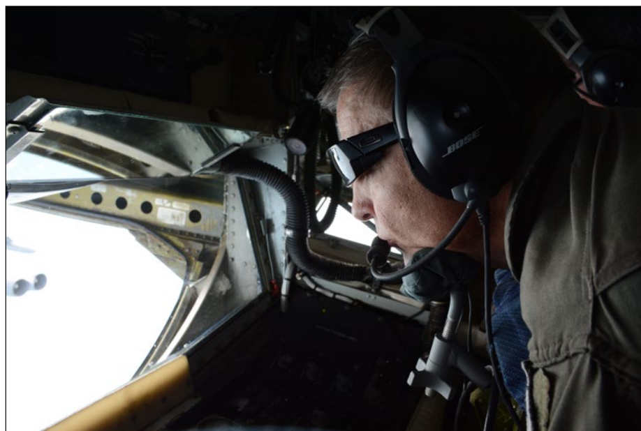
KC-135R aerial refueling is possible due to the efforts of boom operators who lay on their stomach while "flying the boom." Here, Senior Master Sgt. Darby Perrin, 465th Air Refueling Squadron operates the boom while refueling a B-52 Stratofortress at 27,000 feet. (U.S. Air Force photo/Maj. Jon Quinlan)
